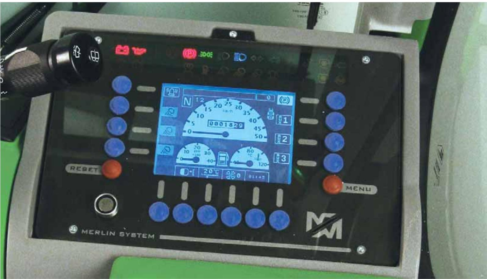
The MERlin system introduces a new way of graphically displaying all machine functions, substituting a lcd display for the traditional instrument cluster to present all necessary information to the driver in a clear and functional manner.
